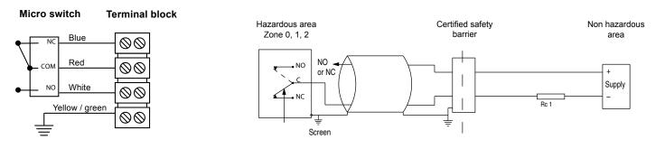
For max. ambient temperature according to temperature classes T5 and T6 refer to technical data on page 1. The installation must be made in an intrinsically safe circuit whose certified electrical safety parameters do not exceed any of the values  $U_{max}$ ,  $I_{max}$  and  $P_{max}$  given in the electrical data on page 1.
